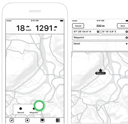
Figure 2.7: Tapping on “Waypoint” will add a new waypoint in the center of the screen – Waypoint editing screen where you can move the waypoint around, manually enter coordinates or rename it
