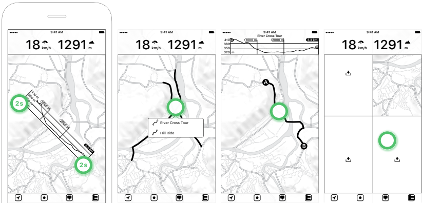
Figure 2.4: Tapping with two fingers for > 2 seconds will show an interactive altitude profile – If multiple tours are overlapping, a tour pop-up is shown – Tapping on a tour will display details and an altitude profile – Tap on the download icon to quickly download missing map data
